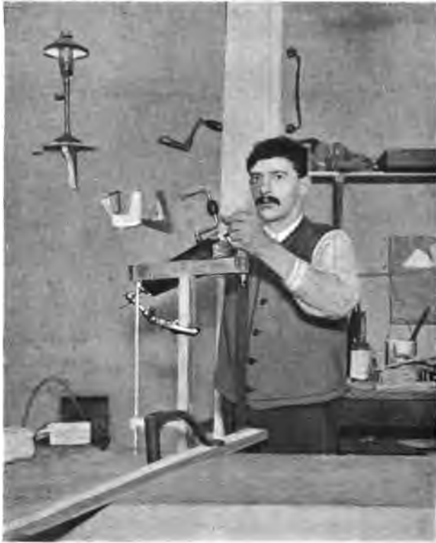
FIG. 132.—One-armed Worker cutting Wood by means of a Rip-saw.
